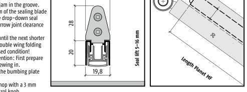
8 Adjustment: adjust the Planet MF in such a way that the sealing blade fits close to the floor when the door is closed. In case of sound absorbing doors: provide by all means a floor rail and a floor separation (e.g. Planet F or Planet BT).
