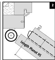
can be shortened flexibly without removal of the Planet seal (shape the door on the bottom). Lift height 20 mm,
