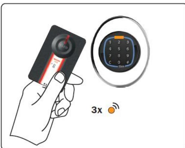
5. At the end of the operation present again the *Master Cards 1* to the device to go out from the *Programming Mode*.
