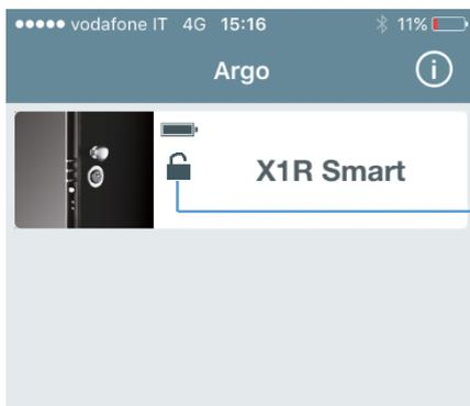
Keeping pressed the *remote opening button*, the lock opens and keeps the latch back. After 7 sec. the *Argo* app will show the *Passage Mode* status (door always open).
