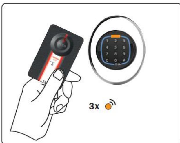
5. At the end of the operation present again the *Master Card 1* to the device to go out the *Programming Mode*.
