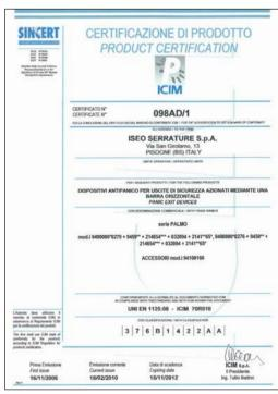
The ICIM certification as per EN1125 is only valid if the operating bars listed in this page are used in conjuction with Iseo locks and striking plates, as indicated in the table.
