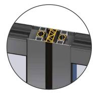
Four-way sealing surfaces in the vertical interlocked structure, including thermal insulation.
