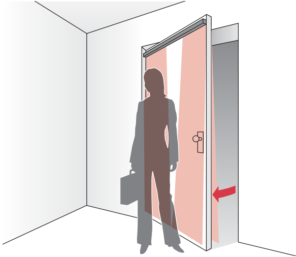
Possible protection of a swing door with Bircher Reglomat sensors.
